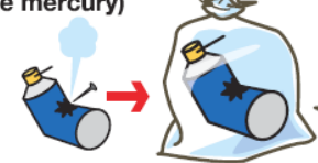
Puncture the containers to release any remaining gas
